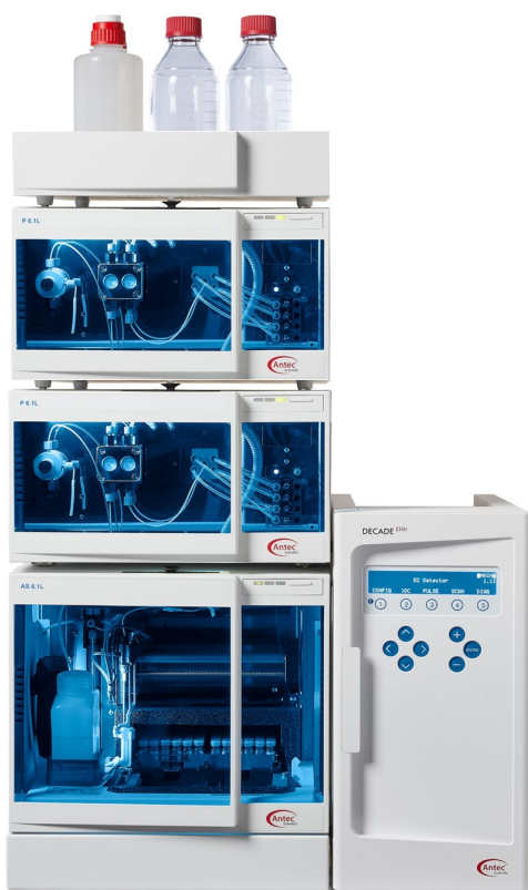
Figure 1: ALEXYS analyzer for Gentamicin.
